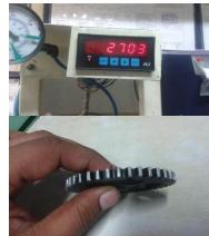
**ROOT CAUSE:** Gear teeth wear out.
